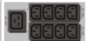
1x IEC C19 outlets 8x IEC C13 outlets
